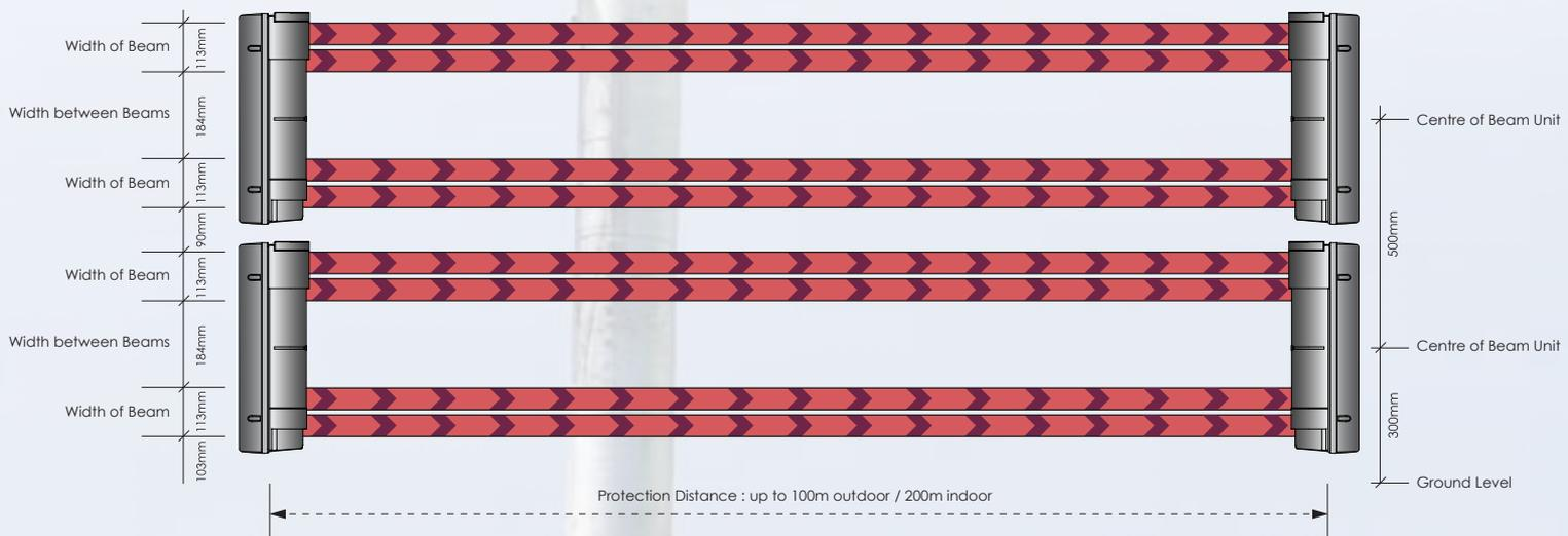
The modular design of the PXB-100ATC sensors ensures that systems can be implemented based on the needs of the application and environment. Sensors can be integrated in a 'tower' configuration to create a high security detection zone of 100m outdoors, to a height of over 8m.
